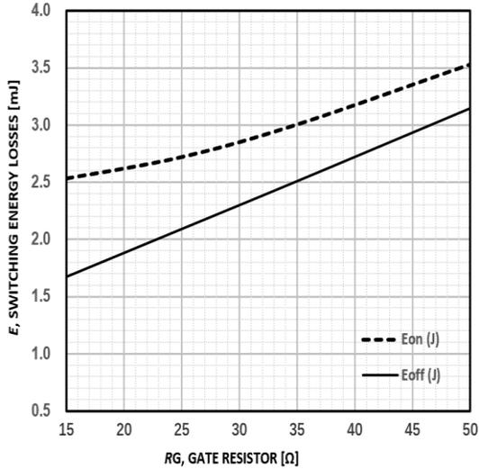
Figure9: Typical energy loss VS. Rg,TC=25°C,
