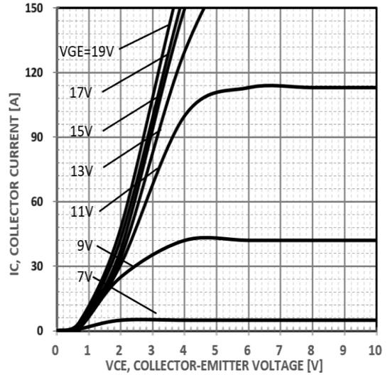
Figure 6. Typical output characteristics
