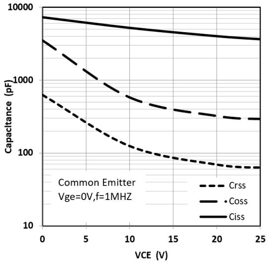
Figure17:Typical capacitance VS. VCE,
