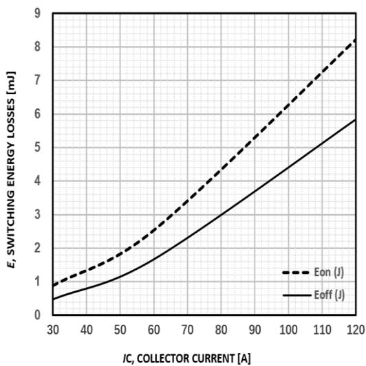
Figure11: Typical energy loss VS. IC, TC=25°C ,
