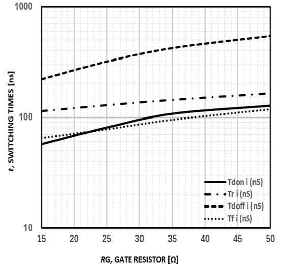
Figure10: Typical switching time VS. Rg,TC=25°C,
