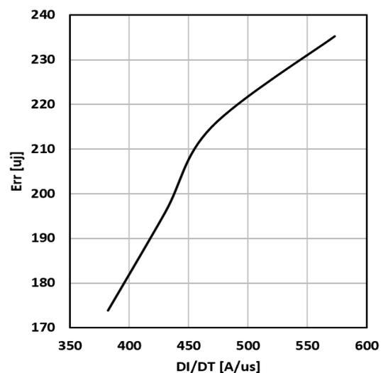
Figure 16. Typical diode Err vs di/dt Tc=25°C
