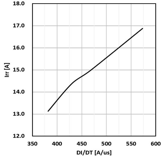
Figure 14. Typical diode Irr vs di/dt Tc=25°C
