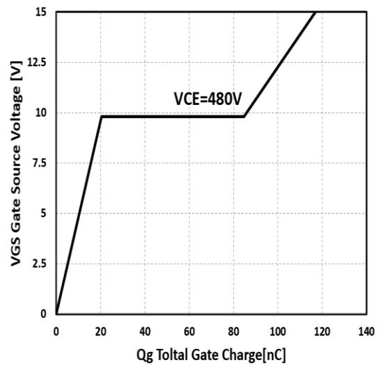
Figure 4: Typical gate charge VS.  $V_{GE}$ ,  $I_C=60\text{A}$
