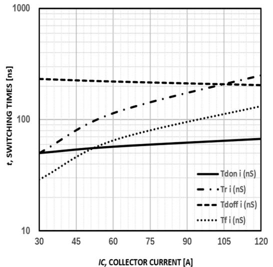
Figure12: Typical switching time VS. IC, TC=25°C ,
