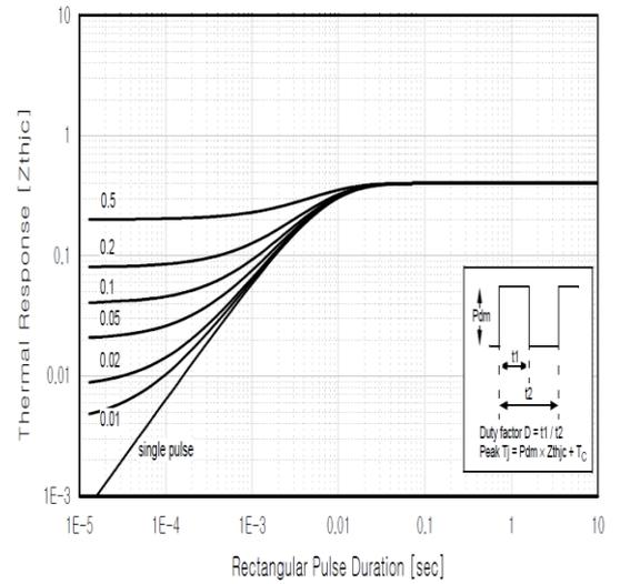
Figure18. normalized transient thermal impedance,
