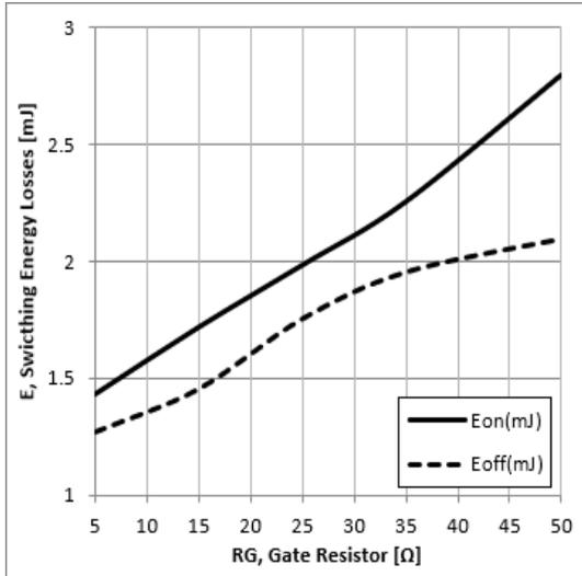
Figure 9: Typical Energy Loss VS. RG, TC=25°C,
