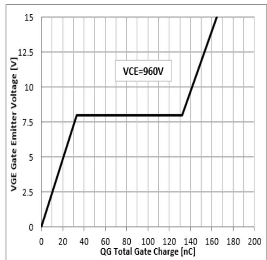
Figure 4: Typical Gate charge VS.  $V_{GE}$ ,  $I_C=30\text{A}$
