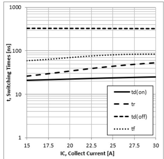
Figure 12: Typical Switching Time VS. IC, TC=25°C,
