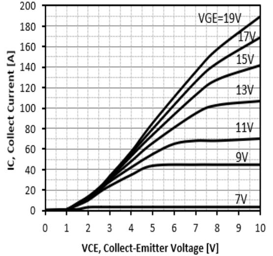
Figure 6: Typical IGBT Output characteristics,
