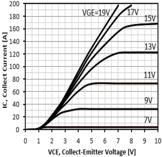
Figure 5: Typical IGBT Output characteristics,
